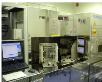
Ultra Precision Flatness measuring system NANOMETRO 300TT for 12" wafer
