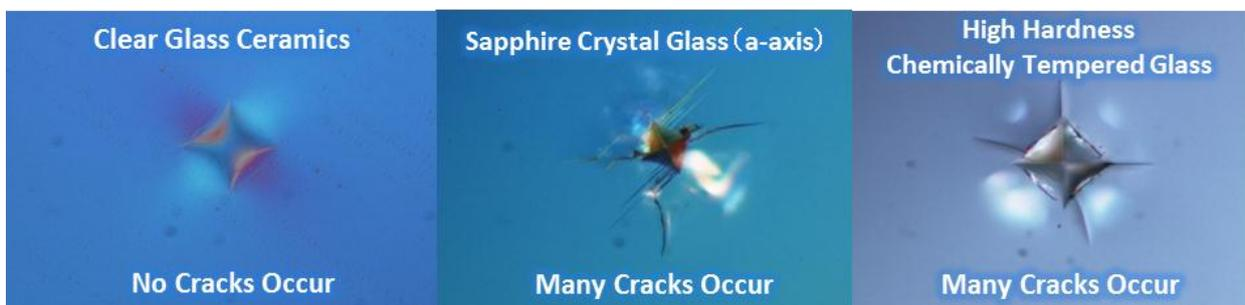
(Pictures when diamond intender is indented at 500gf load according to Vickers Hardness Test.)
